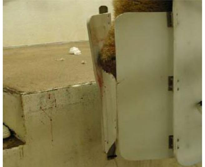
The flexi-reader panels are placed at 45° to each other to de-tune and reduce the read range. As a carcass pushes between the flexi-panels they re-tune, and proximity sensors allow the eartag EID to be read by the pre/post EID blocker. The pre/post EID blocker then checks the EID with a list of previous EID's recorded and only sends the ID if it is a new one.
