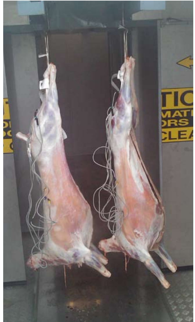
Figure 4 Lamb carcasses being loaded into a prototype air chiller for VFC experiments
