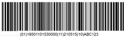
Figure 11: GS1-128 Barcode capturing GTIN, production date and batch/Lot number.
