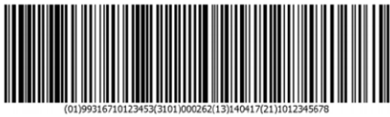
Figure 12: GS1-128 Barcode capturing variable weight GTIN, use of application identifiers (AIs) net weight in kilograms, packaging date and serial number date.
